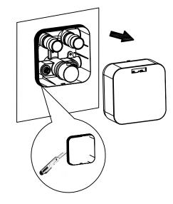
3.After decorating the wall, remove the protective cover and divide the part of the concealed box above the wall.
