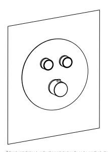
$7. \\ Finish installation, turn the themostatic handle and press the button to turn on the mixer. \\ Check the mixer that working properly.$
