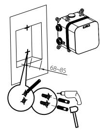
1. According to the picture of mixer instrallation size,dig a suitable hole in the wall (the depth of the wall is 73-86 after decoration). Put the mixer in the suitable location and mark the two fixing holes. Use an electric drill to drill ./7 holes at the mark and insert the expansion rubber particles, and then fix the mixer with self-tapping screws.
