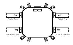
2.Use your own water pipes connections, connect the mixer to the hot and cold water sources by the left hot (red) right cold (blue)(hot and cold water must be connect correctly, otherwise the temperature cannot be adjusted). The water outlet is connected to the required water outlet port respectively(shower head, hand shower, etc) and check any leaks at each connection.
