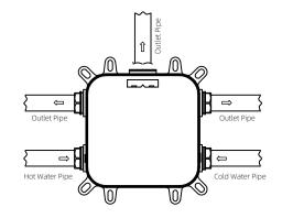
2.Use your own water pipes connections, connect the mixer to the hot and cold water sources by the left hot (red) right cold (blue)(hot and cold water must be connect correctly, otherwise the temperature cannot be adjusted). The water outlet is connected to the required water outlet port respectively(shower head, hand shower, etc) and check any leaks at each connection.
