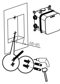
1. According to the picture of mixer instrallation size,dig a suitable hole in the wall (the depth of the wall is 73-86 after decoration). Put the mixer in the suitable location and mark the two fixing holes. Use an electric drill to drill ./7 holes at the mark and insert the expansion rubber particles, and then fix the mixer with self-tapping screws.
