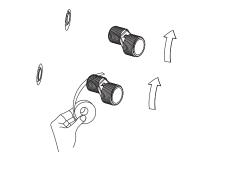
2. After wrapping the eccentric with PTFE tape, please connect with the pre-embedded water oulet pipe connector.
