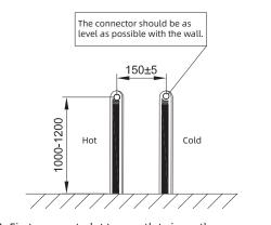
First ensure to let two outlets is on the same level before instrallation and the distance between two water outlets is within the allowable range.Please use the left-hot right-cold connection for the cold and hot water.
