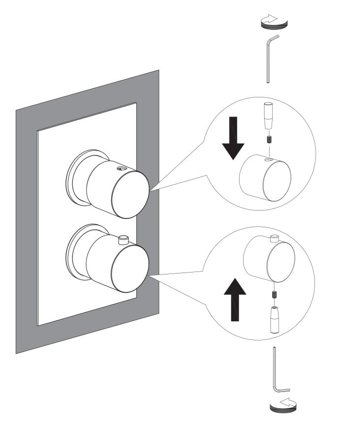
6. Tighten the screws with the Hex Wrench, and install the handle.
