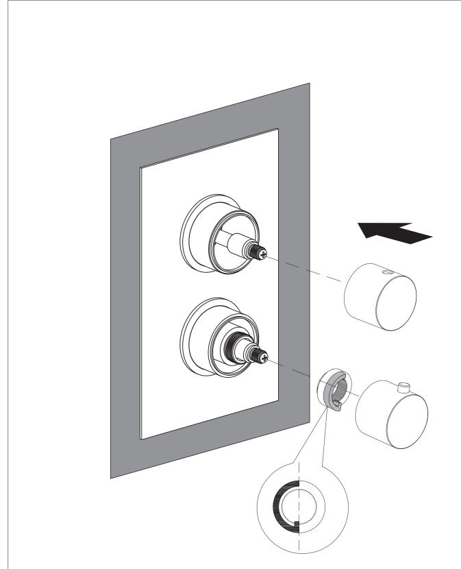
5.Follow the direction from the picture to install the fixed ring, thermostatic handle,switch handle
