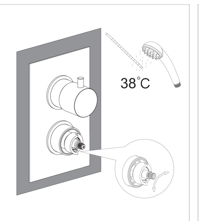
8.Check the temperature difference from the 38°C outlet water (±2°C is Normal phenomenon)Take out the thermostatic handle, turn the thermostatic handle to adjust the temperature and reinstall the thermostatic handle.
