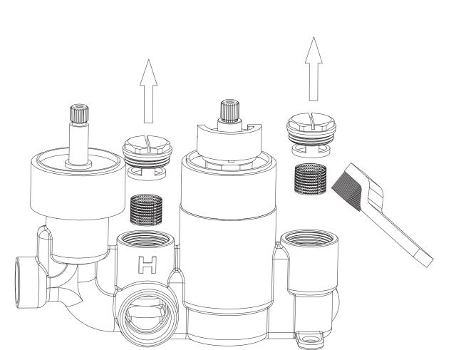
3. When the thermostatic system mail-function, follow the steps below for maintenance: 1) Provide an external force in the hottest / coldest place, Impurities can be washed away. Repeat the above operation to thermo static effect recovery;
