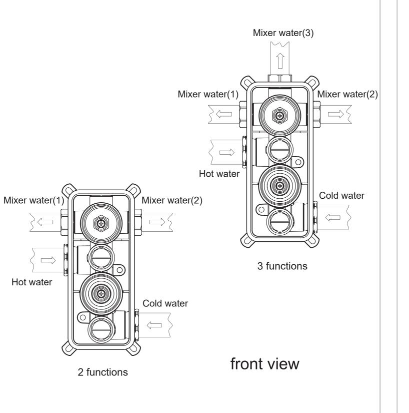
2. Connect the inlet and outlet pipes to the main body according to the instructions in the figure. After marking the position, fix the prc-embedded main body with screws (note the adjustment to ensure that the main body is level).
