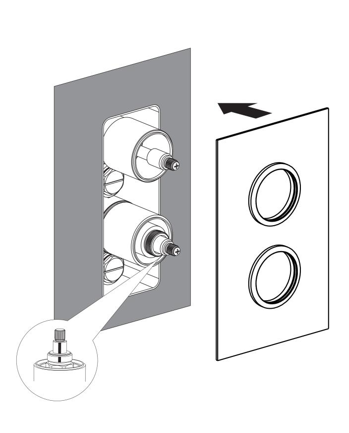
4. Check the thermostatic cartridge is aligned with the line of the handle seat as the factory setting of 38 °C and hang the cover to the main body for fixation.
